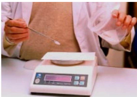
Step 1: Carefully weigh 10 grams of the salt sample to be tested using an electronic open pan micro-balance
