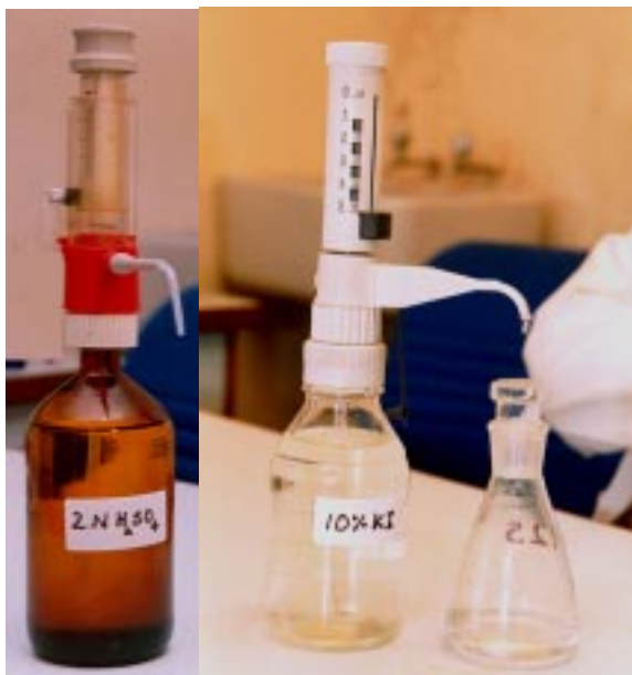
Step 7: Using the automatic dispensers*... (for 2N Sulphuric Acid on the left and for 10% Potassium Iodide on the right)...
