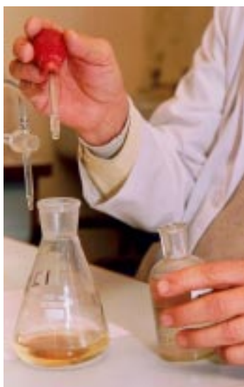
Step 18: Add 2 drops of the 1% starch solution...
